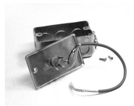
The splice point should stay inside the junction box. That is, you want to feed the long run of cable into the box rather than pulling the pigtail out. Electro-Mech provides a strain relief on one side of the junction box to secure the cable. You may choose to connect conduit directly to the junction box, in which case the strain relief will not be needed. The junction box is designed to accept 3/4-inch conduit fittings.
